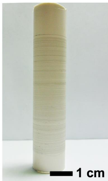
Figure S5. Photograph of a roll of a continuous HPF after an oxygen plasma treatment.
