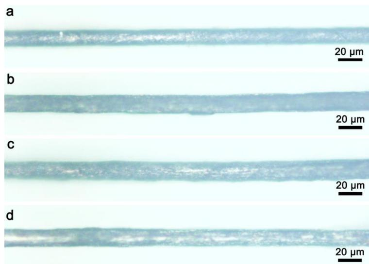
**Figure S4.** Optical microscopic images of a CNT/RGO composite fiber. The deposition time for this CNT/RGO fiber was 180 s. Four sections were taken from a 1 m composite fiber at four points: 20 cm, 40 cm, 60 cm and 80 cm. Each section had a length of 5 mm and was observed under an optical microscope. The four sections of the CNT/RGO composite fiber had a uniform diameter and morphology.
