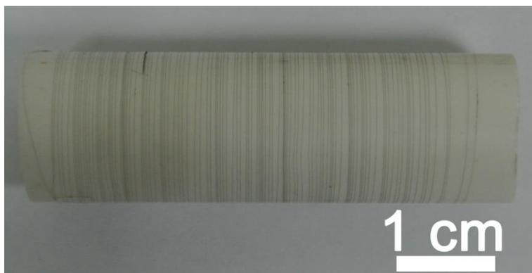
**Figure S8.** Photograph of a 5 m-long fiber-shaped supercapacitor wrapped on a plastic tube. The supercapacitor was made by twisting two CNT/RGO composite fibers.
