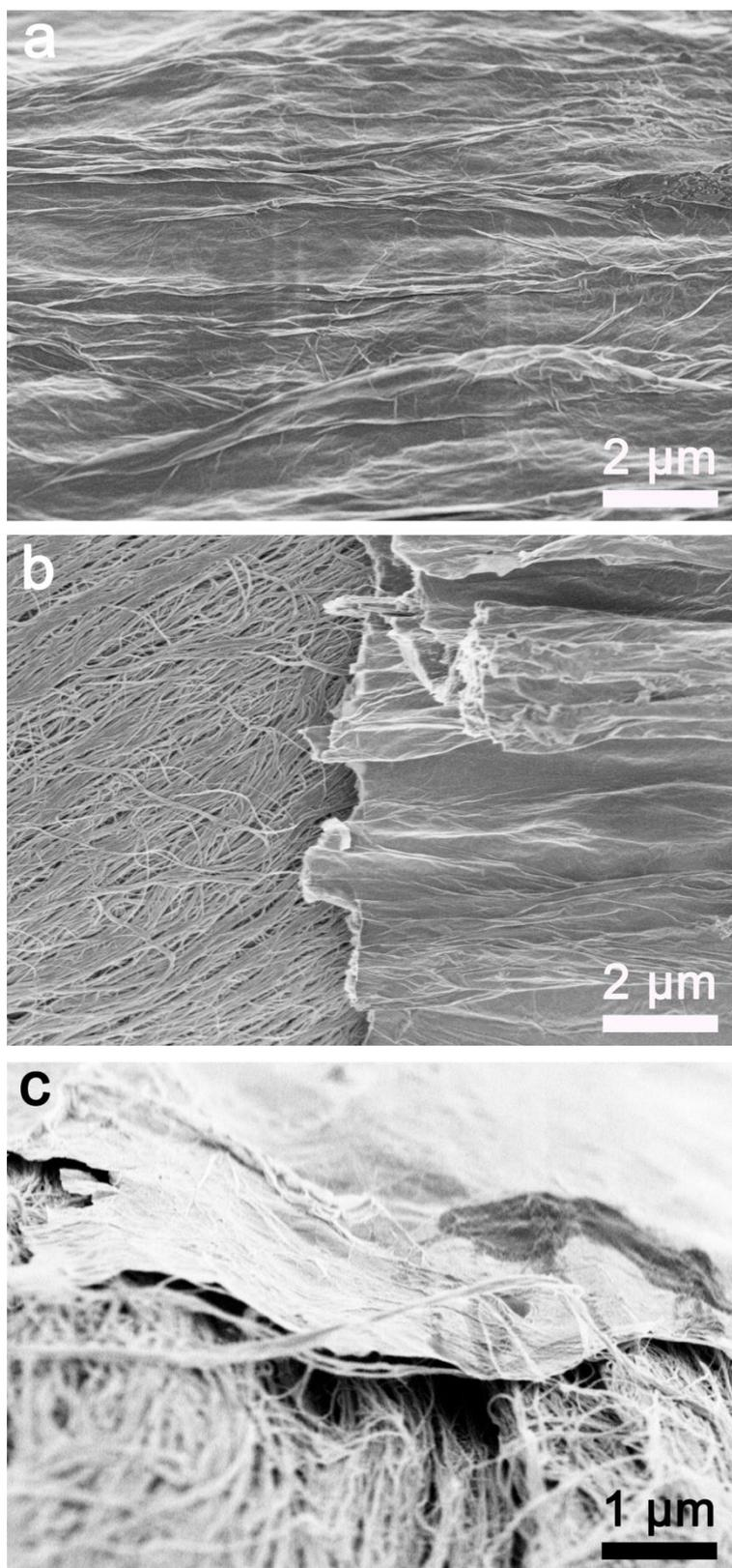
**Figure S2.** **a.** High magnification SEM image of the CNT/RGO composite fiber. Part of RGO on the surface was removed to expose the CNTs. **b** and **c.** High magnification SEM images of the RGO layer wrapped on the CNT fiber. The deposition time for this CNT/RGO composite fiber was 120 s.
