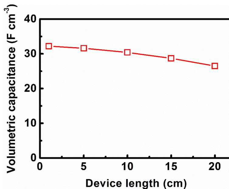
**Figure S27.** Volumetric capacitances of fiber-shaped supercapacitors in different lengths. The supercapacitors were continuously produced and were assembled from CNT/RGO composite fibers under a deposition time of 180 s. The current density was 1240 mA cm<sup>-3</sup>.
