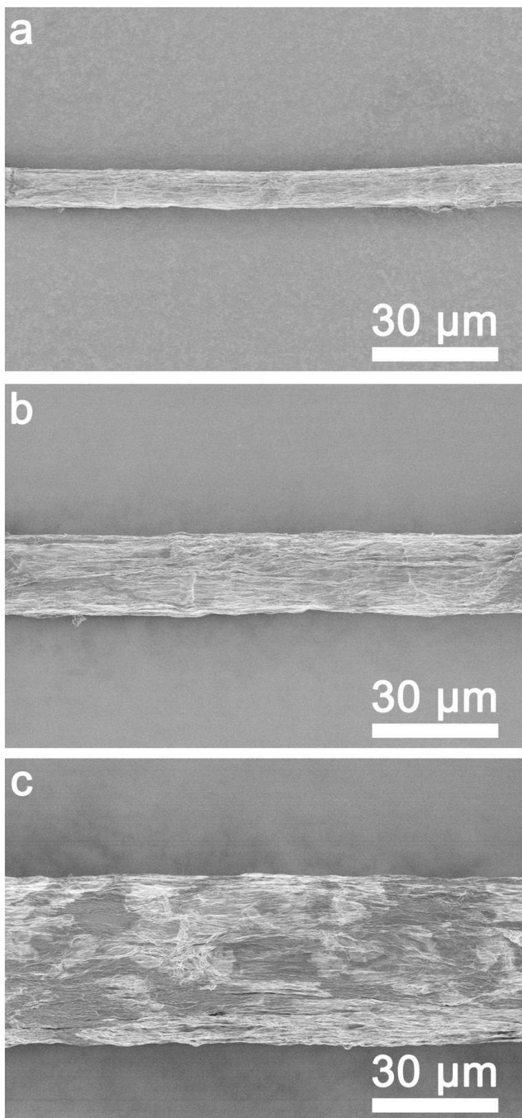
**Figure S6.** SEM images of CNT/RGO composite fibers of different diameters. The initial diameters of CNT fibers were 10  $\mu\text{m}$  (a), 20  $\mu\text{m}$  (b) and 35  $\mu\text{m}$  (c). The deposition time for these samples was 180 s.
