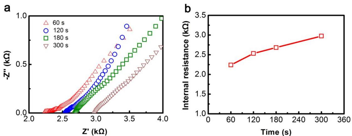
**Figure S18.** **a.** Electrochemical impedance spectra of fiber-shaped supercapacitors made from CNT/RGO composite fibers that were prepared under different deposition time. **b.** Internal resistances that derived from the horizontal intercepts of **a.** The electrochemical impedance measurement was conducted from 10 mHz to 1 MHz with a voltage amplitude of 5 mV.
