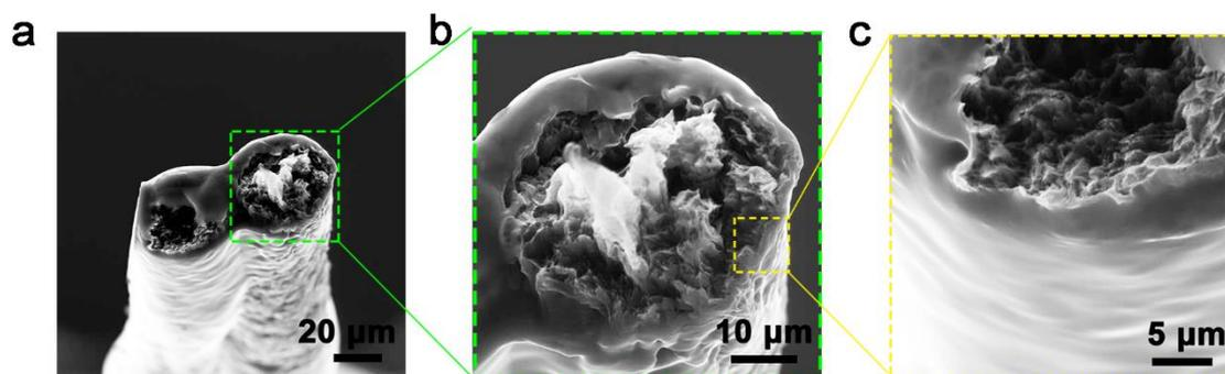
**Figure S7.** Cross-sectional SEM images of fiber-shaped supercapacitor made from CNT/RGO composite fibers by a localized view of the interface between the electrolyte and electrode. **a.** The fiber-shaped supercapacitor. **b.** Magnified image of **a**, displaying a CNT/RGO composite fiber externally coated with electrolyte. **c.** Magnified image of **b**. The fiber-shaped supercapacitor was broken up in a liquid nitrogen.
