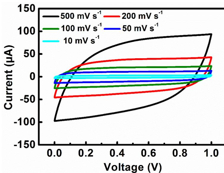
**Figure S15.** Cyclic voltammograms of fiber-shaped supercapacitors based on CNT/RGO composite fibers at increasing scan rates. The deposition time for CNT/RGO composite fiber here was 180 s.
