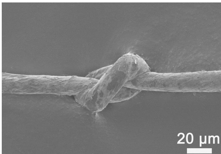
**Figure S5.** SEM image of a knotted CNT/RGO composite fiber. The deposition time for this sample was 180 s.
