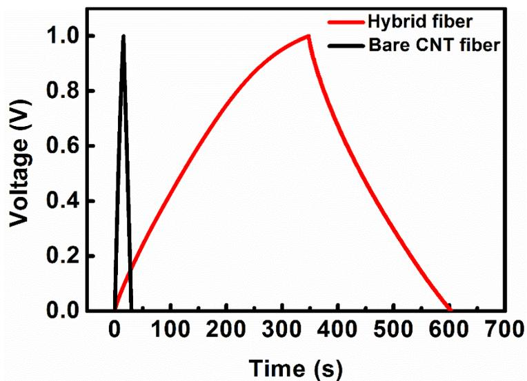
**Figure S14.** Galvanostatic charge-discharge curves of fiber-shaped supercapacitors based on bare CNT and CNT/RGO composite fibers at  $62 \text{ mA cm}^{-3}$ . The deposition time for CNT/RGO composite fiber here was 180 s.
