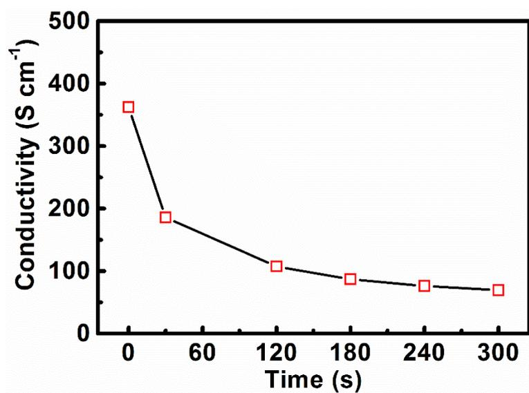
**Figure S13.** Electrical conductivities of CNT/RGO composite fibres prepared at different depositing times. The original diameter of CNT fiber was 20  $\mu\text{m}$ .
