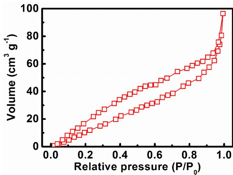
**Figure S3.** Nitrogen adsorption–desorption isotherm of RGO sheets. The RGO samples were peeled from the CNT/RGO composite fibers.
