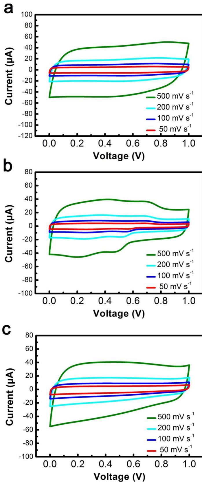
**Figure S21.** Cyclic voltammograms of fiber-shaped supercapacitors based on CNT/ $\text{MnO}_2$  composite fibers (a), CNT/PANI composite fibers (b) and CNT/PPy composite fibers (c).
