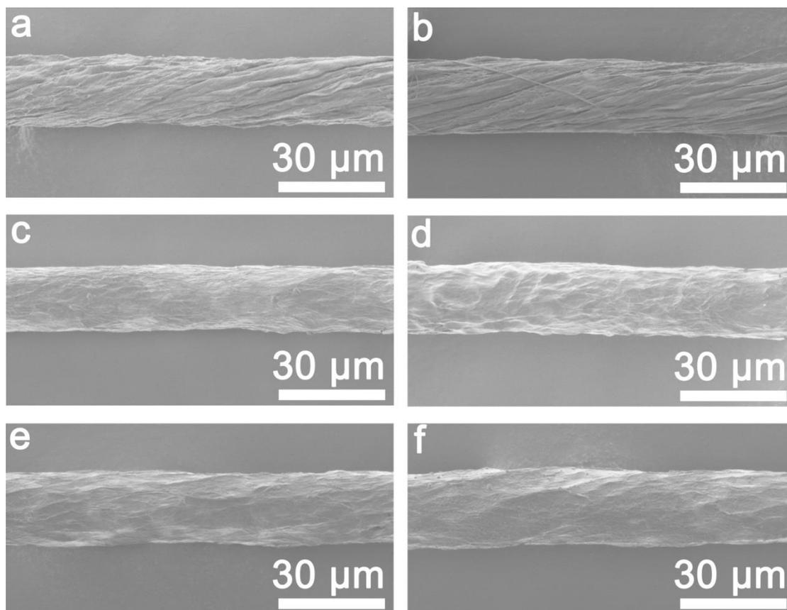
**Figure S9.** SEM images of CNT/RGO composite fibers prepared under different deposition time. **a.** 30 s. **b.** 60 s. **c.** 120 s. **d.** 180 s. **e.** 240 s. **f.** 300 s. The original diameter of CNT fiber was 20  $\mu\text{m}$ .
