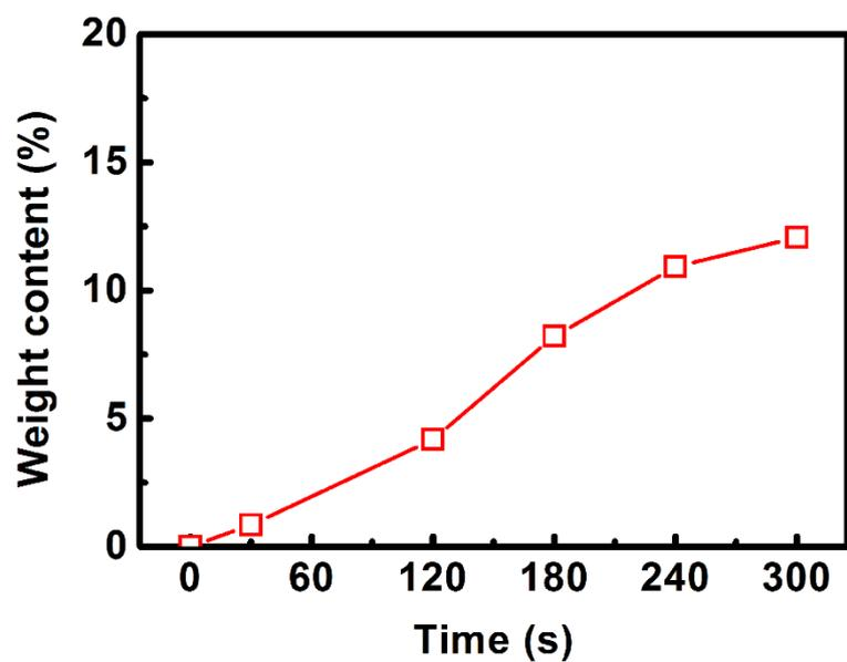
**Figure S10.** The weight content of RGO in CNT/RGO composite fibers prepared under different deposition time. The masses of CNT fibers and CNT/RGO composite fibers were defined by an element analytical balance.
