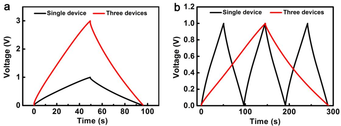
**Figure S26.** Galvanostatic charge-discharge curves of single supercapacitor and three supercapacitors being connected in series (**a**) and in parallel (**b**). The current density for charge and discharge was  $310 \text{ mA cm}^{-3}$ . The supercapacitor was made from CNT/RGO composite fibers.
