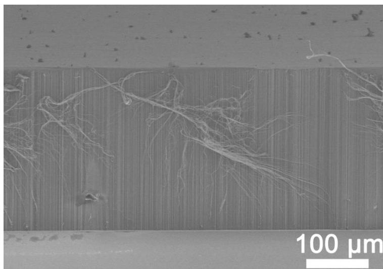
**Figure S1.** SEM image of the cross-sectional view of a spinnable CNT array. The CNT array was grown on a silicon wafer by chemical vapor deposition.
