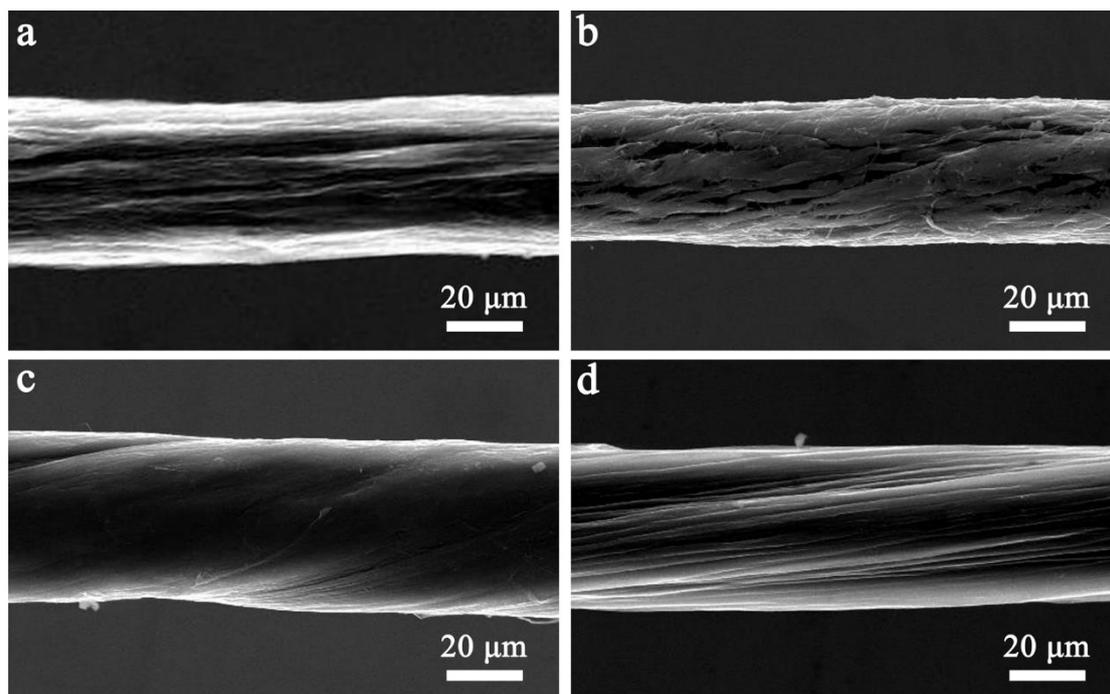
**Figure S25.** SEM images of different composite fibers after bending for 1000 times. The bending angle was  $180^\circ$  and the bending radius was 0.5 cm. **a.** CNT/RGO composite fiber. **b.** CNT/MnO<sub>2</sub> composite fiber. **c.** CNT/PANI composite fiber. **d.** CNT/PPy composite fiber.
