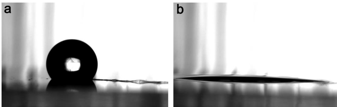
**Figure S16.** The hydrophilicity of CNT and CNT/RGO composite. The contact angle measurements were conducted on planar samples. **a.** CNT sheets. **b.** CNT/RGO composite sheets. The CNT/RGO composite sheets were prepared through the same electrochemical deposition method. The deposition time was 180 s. The contact angles of CNT and CNT/RGO composite are  $137^\circ$  and  $10^\circ$ , respectively.
