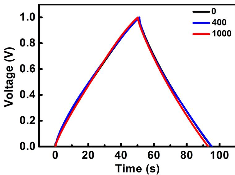
**Figure S23.** Galvanostatic charge-discharge curves of a fiber-shaped supercapacitor before and after being bent to 180 ° for 400 and 1000 cycles. The supercapacitor was made from CNT/RGO composite fibers. The current density for charge and discharge was 310 mA cm<sup>-3</sup>.
