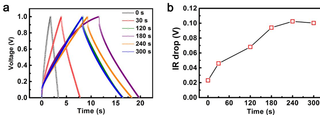
**Figure S19. a.** Galvanostatic charge-discharge curves of fiber-shaped supercapacitors made from CNT/RGO composite fibers that were prepared under different deposition time. The current density for charge and discharge was  $2500 \text{ mA cm}^{-3}$ . All the samples for electrochemical tests had the same length. **b.** The relation of voltage drops induced by internal resistance with deposition time. The IR drops were defined from charge-discharge curves in **a.**
