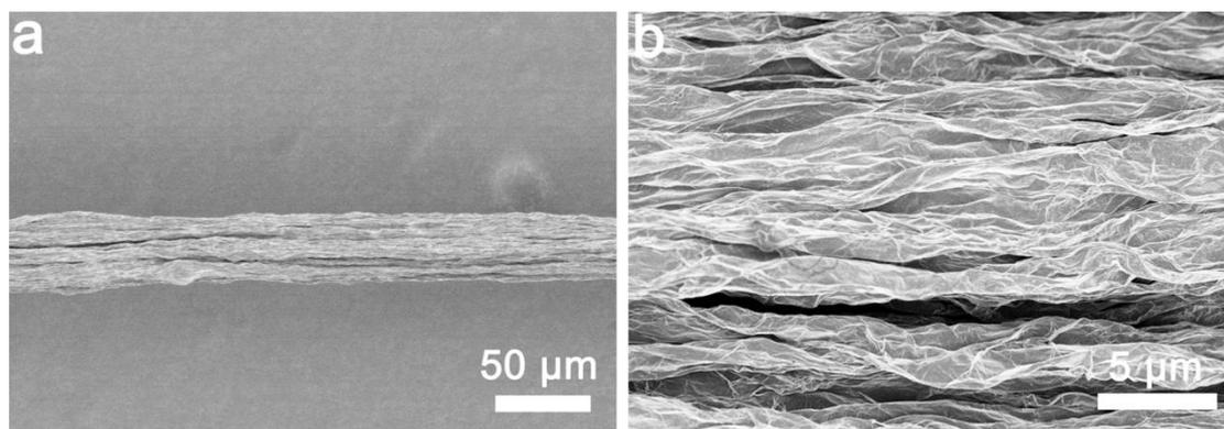
**Figure S20.** SEM images of graphene fibers at low (**a**) and high (**b**) magnifications. The graphene fiber was prepared through wet-spinning method (C. Gao et al., *Adv. Mater.* 2013, 25, 188.) and had a diameter of 40  $\mu\text{m}$ . The conductivity of the graphene fiber was  $48.9 \text{ S cm}^{-1}$ .
