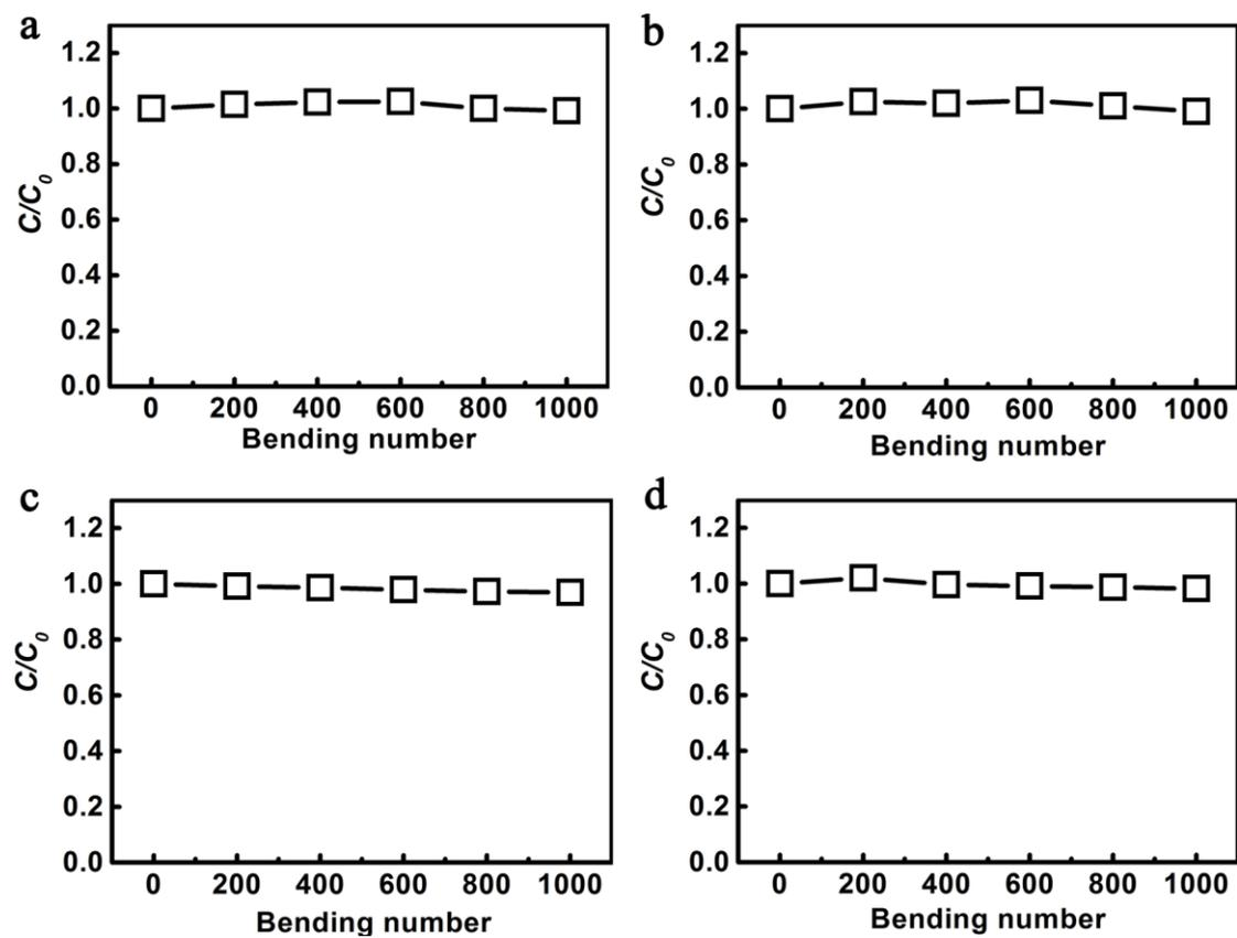
**Figure S24.** Dynamic bending tests of fiber-shaped supercapacitors made from CNT/RGO composite fibers (a), CNT/MnO<sub>2</sub> composite fibers (b), CNT/PANI composite fibers (c) and CNT/PPy composite fibers (d). The bending angle was 180°.
