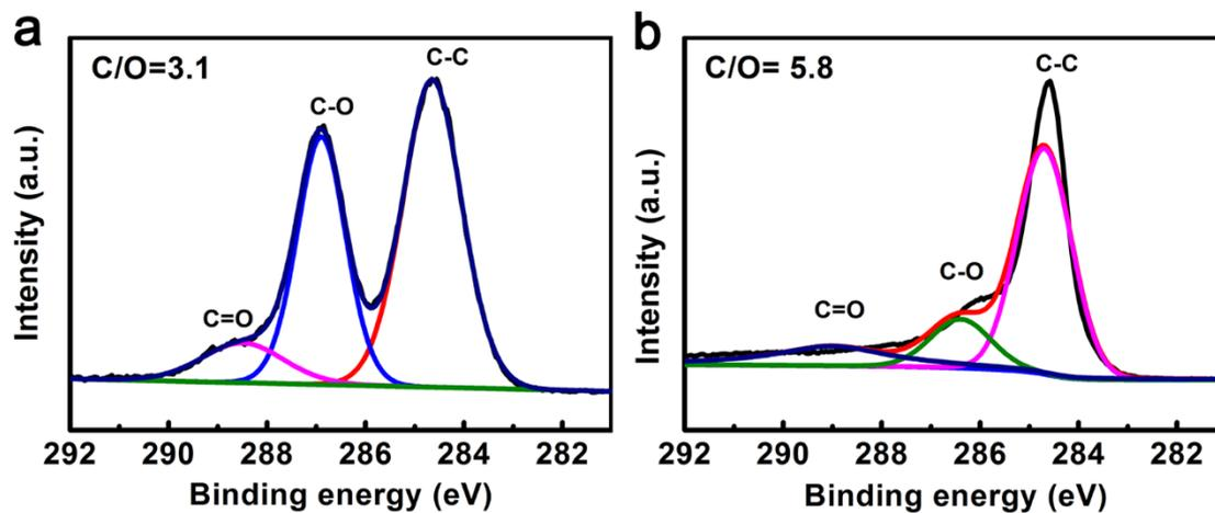
**Figure S12.** X-ray photoelectron spectra of CNT/GO composite fiber (a) and CNT/RGO composite fiber (b). The deposition time for the CNT/RGO composite fiber was 180 s. The carbon/oxygen ratio was increased from 3.1 to 5.8 after reduction, indicating that the GO was partially reduced during the process.
