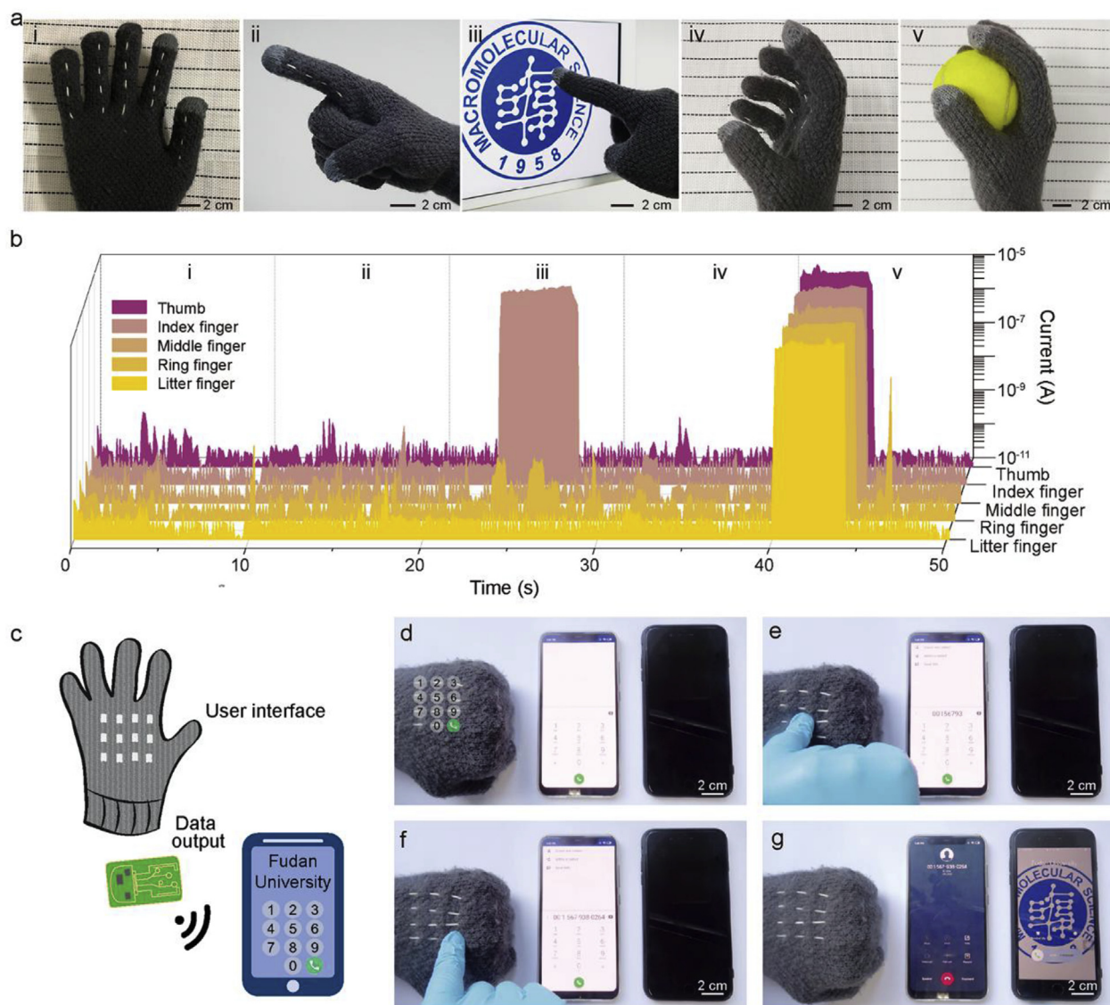
Fig. 4. | Demonstration of the TST being integrated into a smart glove. a , Optical images of a smart glove integrated with the TST on the five fingers, detecting physical contacts under different gesticulations, i.e., (i) open hand, (ii) pointing, (iii) touching, (iv) gripper and (v) grasping. b , The variation of current for each sensor on the glove during executing different gesticulations. c–g , Schematic illustration and optical images of a smart glove integrated with a TST on the back of hand and served as a user interface to control a cell phone.
