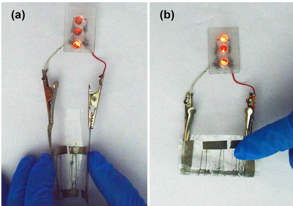
**Figure S8.** Photographs of a flexible fiber supercapacitor to power three LEDs when it was bent to an angle of  $180^\circ$  in parallel **(a)** and perpendicular **(b)** directions relative to the length of the fiber supercapacitor.
