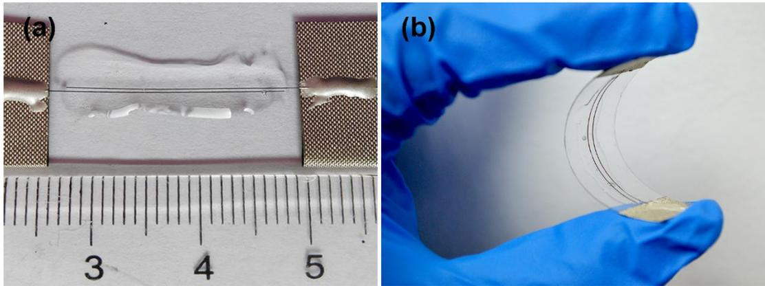
**Figure S4.** a) Photograph of a fiber supercapacitor on glass substrate. b) Photograph of a flexible solid-state fiber supercapacitor.
