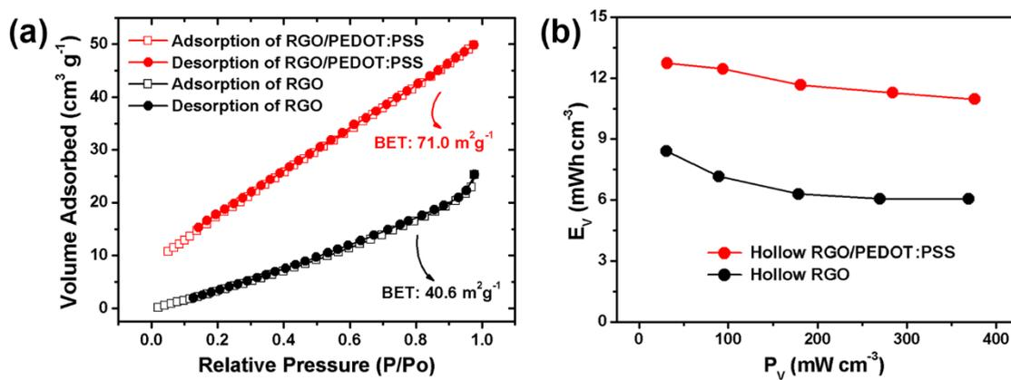
**Figure S6.** a) Nitrogen adsorption-desorption isotherms of HCFs and HPFs. b) Ragone plot of the fiber supercapacitors based on the volume of single fiber.
