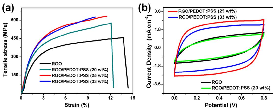
**Figure S3.** a) Typical stress-strain curves of hollow RGO fibers obtained with increasing PEDOT:PSS weight percentages. b) CV curves of the hollow RGO fiber-based supercapacitors obtained with increasing PEDOT:PSS weight percentages.
