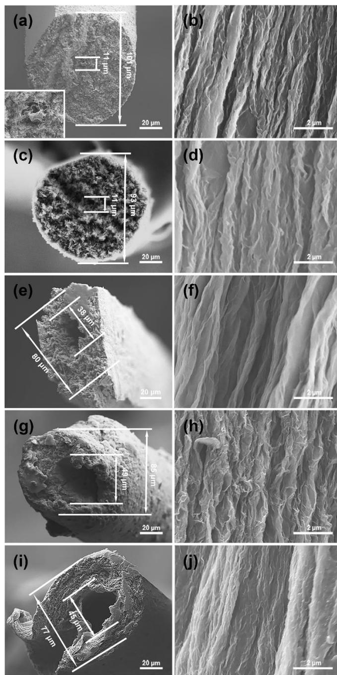
**Figure S1.** SEM images of HPFs without (a, b) and with increasing PEDOT:PSS weight percentages from 10% (c, d), 20% (e, f) and 25% (g, h) to 33% (i, j). The left and right columns correspond to top and side views, respectively. The diameter ratios of the inner to the outer are approximately 11%, 12%, 47%, 58% and 59% for both HPFs and HCFs with increasing PEDOT:PSS weight percentages from 10% to 33%.
