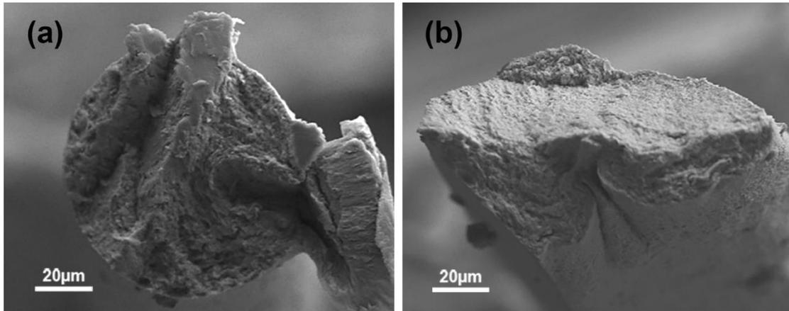
**Figure S2.** a) Cross-sectional SEM image of a solid RGO/PEDOT:PSS composite fiber. b) Cross-sectional SEM image of a solid RGO fiber.
