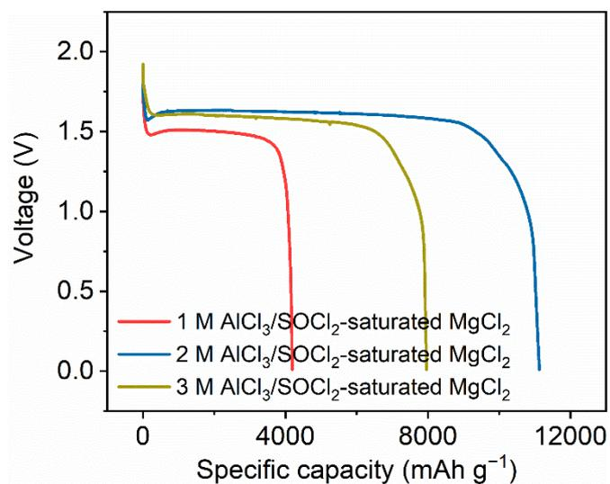
**Figure S3.** The discharging profiles of Mg/SOCl<sub>2</sub> batteries using different electrolytes comprised of increasing AlCl<sub>3</sub> concentrations (1, 2 and 3 M) with the addition of excess MgCl<sub>2</sub> (0.4, 0.8 and 1.2 M) for saturation. Current density, 100 mA g<sup>-1</sup>.
