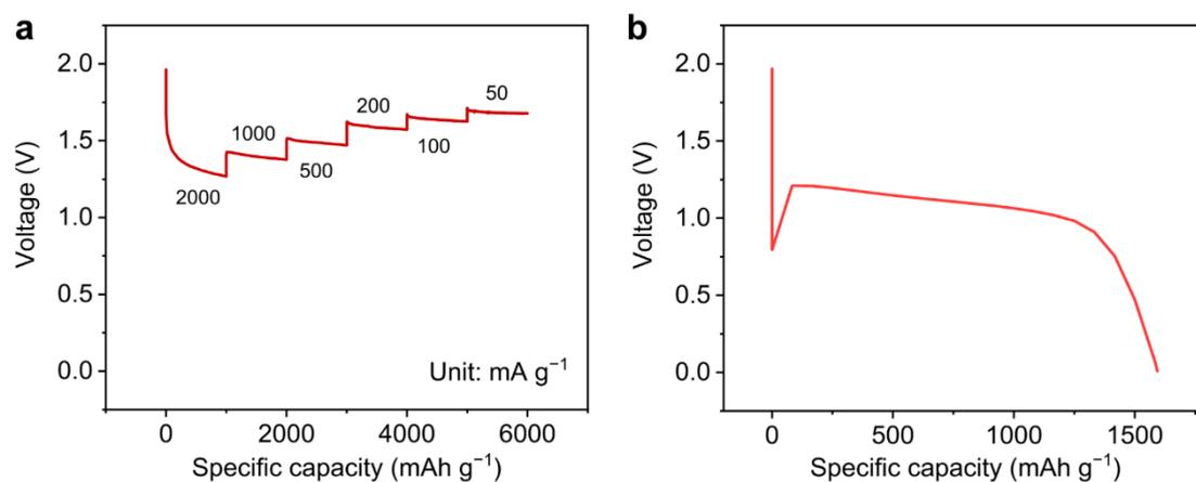
**Figure S6.** a) The discharging profile of a Mg/SOCl<sub>2</sub> primary battery with different discharge current densities from 2,000 to 50 mA g<sup>-1</sup>. b) Galvanostatic discharge curve of a Mg/SOCl<sub>2</sub> primary battery at the current density of 10,000 mA g<sup>-1</sup> at 50 °C.
