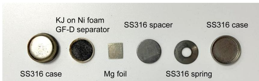
**Figure S12.** Photograph of the disassembled components from a fully discharged Mg/SOCl<sub>2</sub> primary battery.
