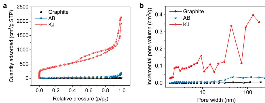
**Figure S5.** a) Nitrogen adsorption-desorption isotherms of graphite, AB and KJ using Brunauer-Emmett-Teller (BET) method. b) Pore size distribution derived from the adsorption branch by the Barrett-Joyner-Halenda (BJH) method.
