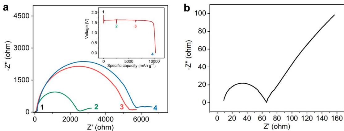
**Figure S7. a)** EIS measurement of a Mg/SOCl<sub>2</sub> primary battery at a variety of discharge states as indicated in the discharging curve of the inset. **b)** EIS measurement of a Mg/SOCl<sub>2</sub> primary battery before discharge.
