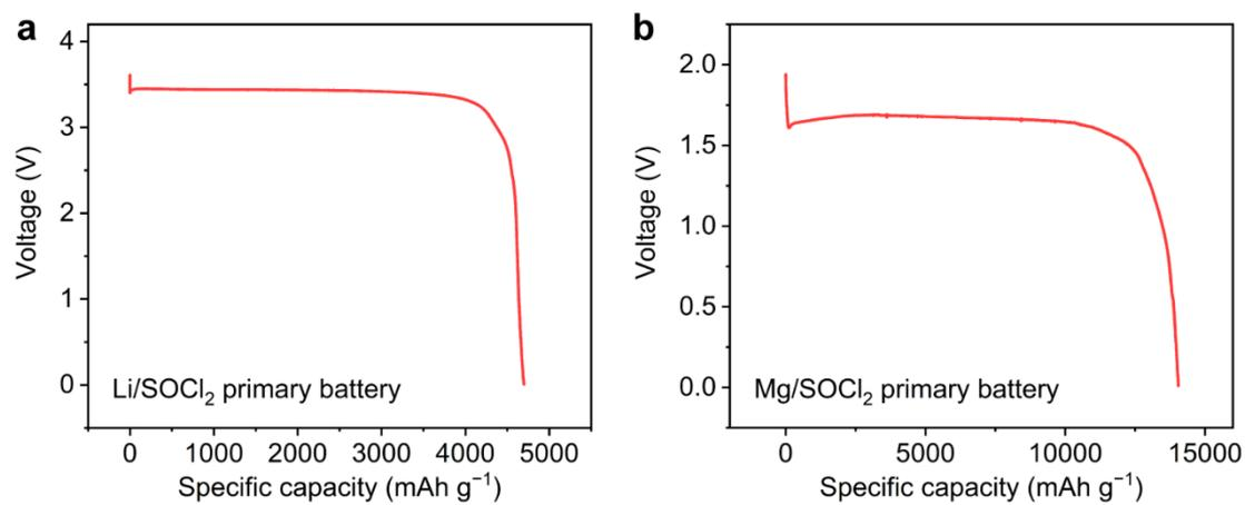
**Figure S1. a, b)** Galvanostatic discharge curves of Li and Mg/SOCl<sub>2</sub> primary batteries at the current density of 50 mA g<sup>-1</sup>, respectively.
