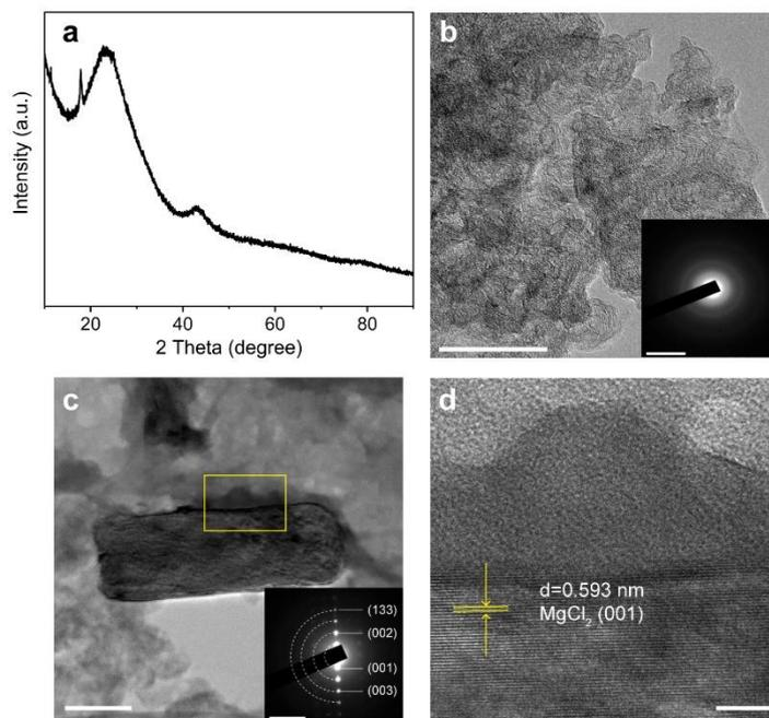
**Figure S9.** **a, b)** XRD pattern and TEM image of the KJ, respectively. Inset in **b**, SAED pattern. Scale bar in **b**, 50 nm. Inset, 1/5 nm. **c, d)** TEM and HRTEM images of the KJ after discharge. Scale in **c**, 100 nm. Inset, 1/5 nm. Scale bar in **d**, 10 nm.
