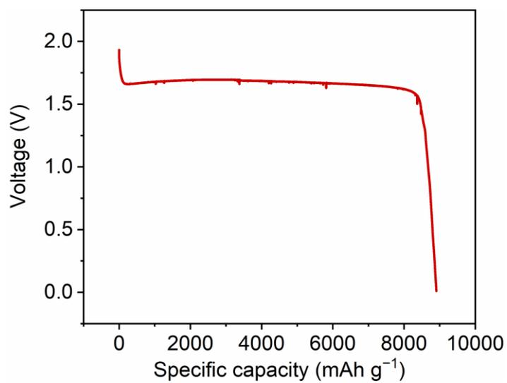
**Figure S8.** Galvanostatic discharge curve of the Mg/SOCl<sub>2</sub> primary battery with a cathode mass loading of 2–3 mg cm<sup>-2</sup> at the current density of 50 mA g<sup>-1</sup>.
