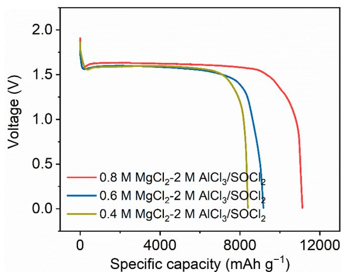
**Figure S4.** The discharging profiles of Mg/SOCl<sub>2</sub> primary batteries using different electrolytes comprised of increasing MgCl<sub>2</sub> concentration (0.4, 0.6 and 0.8 M) with the same AlCl<sub>3</sub> concentration of 2 M. Current density, 100 mA g<sup>-1</sup>.
