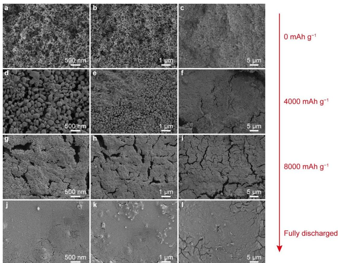
**Figure S10.** SEM images of the discharge products on KJ cathode at different discharge depths. The discharge current density is 100 mA g<sup>-1</sup>.
