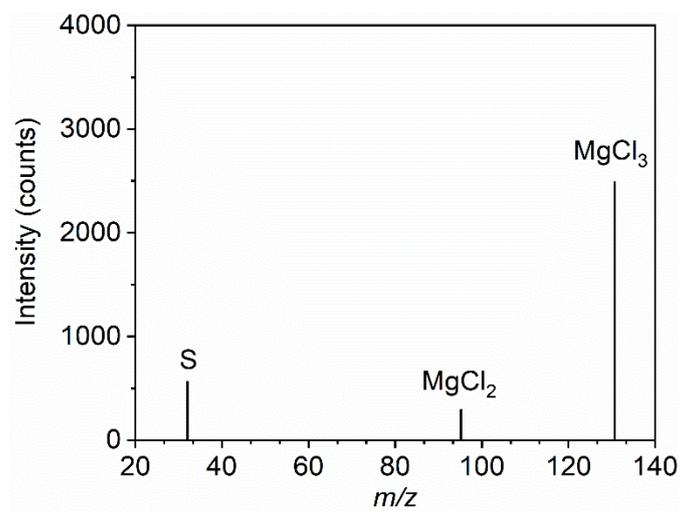
**Figure S11.** TOF-SIMS spectra probing the MgCl<sub>3</sub>, MgCl<sub>2</sub> and S secondary ion fragments from a fully discharged KJ cathode.
