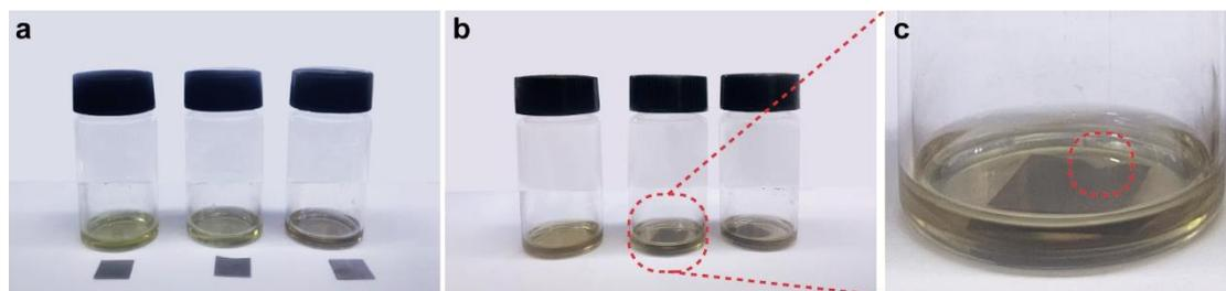
**Figure S2.** a, b) Mg anodes before and after immersing in a variety of electrolytes (left to right: HC-A-SOCl<sub>2</sub>, A-SOCl<sub>2</sub>, A-M-SOCl<sub>2</sub>) overnight, respectively. c) Enlarged photograph from b indicates the Mg metal corrosion in A-SOCl<sub>2</sub> electrolyte.
